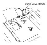
Figure 4-2 Dump Valve Control
